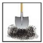
Place PAR in the hole in 3in layers, tamping each layer area until firm. The last layer of PAR is to be 25% higher than the finished level.
