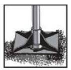
Compact the PAR with a tamper, roller or by driving over it until the desired level is obtained.
