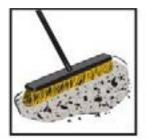
Clean all loose debris or chunks using a stiff broom or a blower to achieve a sound bonding surface.
